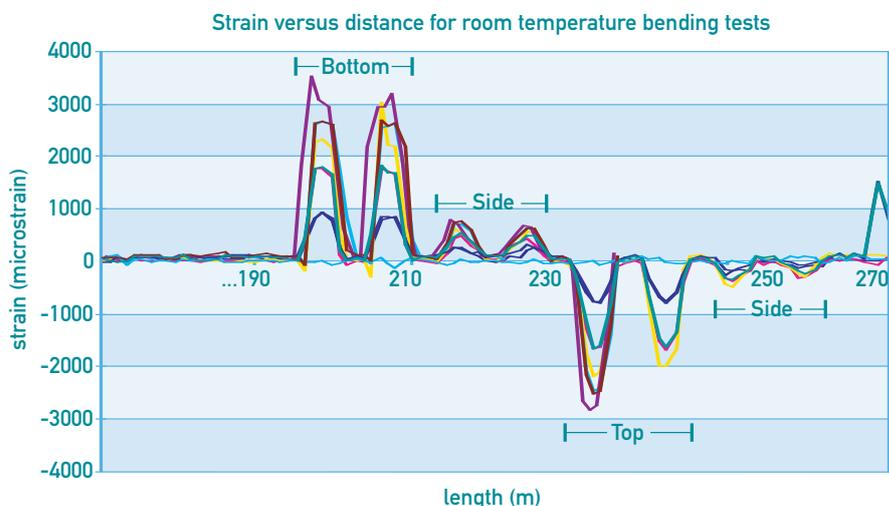
**RESULTS:** The DTSS measured the full distribution of tensional, compressional and bending strains with a 1m spatial resolution. The DTSS detected the elastic limit of the
