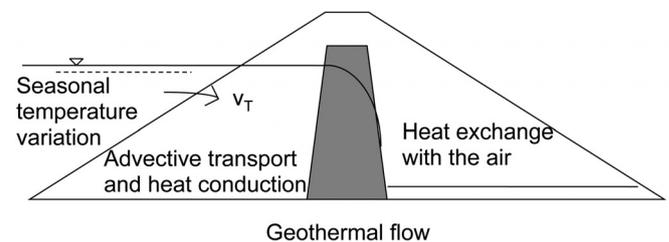
Figure 2 | Basic thermal processes in an embankment dam
