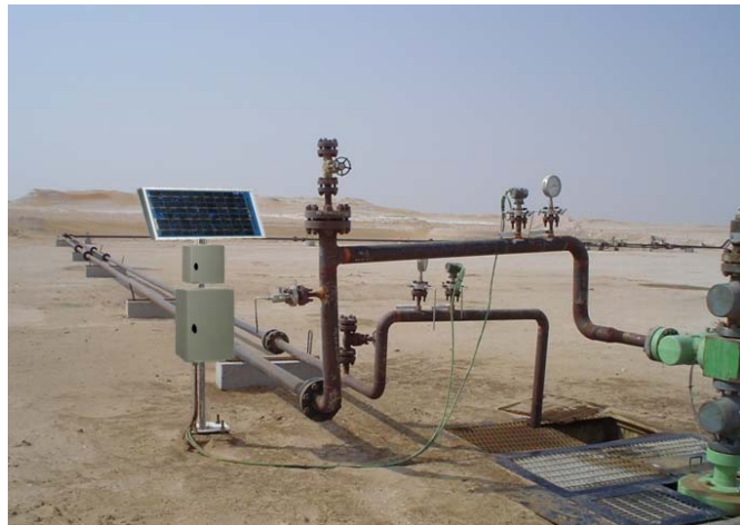
The SensorNet Oryx DTS – a powerful remote logging DTS unit
